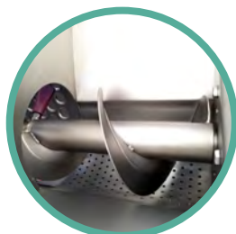
Loading hopper filter
